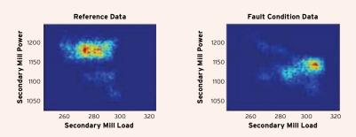
Monitoring of an autogenous mill on an industrial concentrator plant
