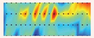
Prognostic monitoring of wall temperatures for a metallurgical furnace
