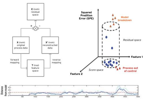
Figure 3: Monitoring the model prediction error in an appropriately constructed feature space enables advance warning of process upsets.
