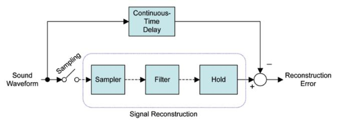
The YY filter design process mathematically optimizes the filter to ensure that the reconstruction error across a desired frequency range-not determined solely by the Nyquist frequencyis less than a design parameter. This is a sampled-data H<sub>w</sub> control problem.
