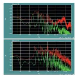
Fast Fourier transforms (0-20 kHz) of an analog record (top) and CD reproduction (bottom). The green trace is the FFT; the red trace is the peak FFT value over the past 10 seconds. The record exhibits a range that extends well beyond 20 kHz; the CD has a sharp cutoff at 20 kHz. (The traces are not from the same sound.)
