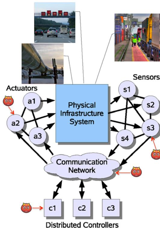
Cyber attacks on CPS control elements can result in the loss of availability (denial-of-service attack) and/or integrity (deception attack) of safety-critical measurement and control data.
