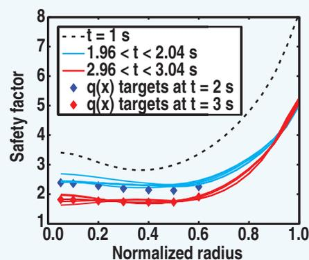
Experimental results of controller capability to track changes in the target safety-factor profile  $q(x)$  (at  $t = 2$  and 3 sec), from an arbitrary value (at  $t = 1$  sec)
