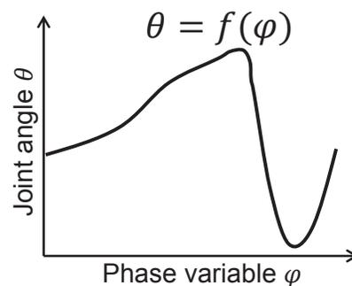
Conceptual diagram of shift from sequential control to virtual constraint control, where joint patterns are characterized by continuous functions of a mechanical phase variable
