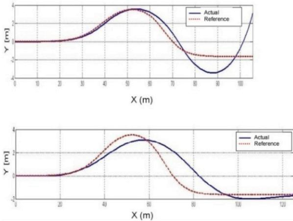
The reference (red) and actual (blue) DLC trajectories on snow at 55 kph are shown for a fixed PID gain steering robot designed for asphalt surfaces (top) and for an MPC system that incorporates vehicle stability state constraints (bottom). Neither car has electronic stability control. The MPC anticipates that aggressive steering could lead to loss of traction, thus trading off its initial tracking error for future gains and successful completion of the DLC maneuver.
