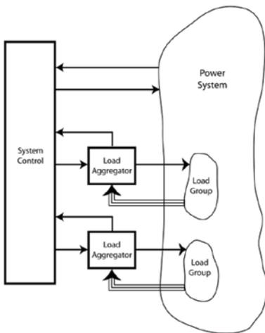
A hierarchical control structure for integrating nondisruptive load control into power system operation
