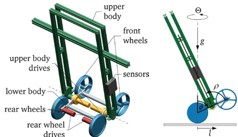
CAD model of the SCD (above left) with main degrees of freedom (above right): position  $l$ , lower body angle ( $\theta$ ), upper-lower body angle ( $\rho$ ), yaw angle ( $\Theta$ ), and gravitational acceleration  $g$
