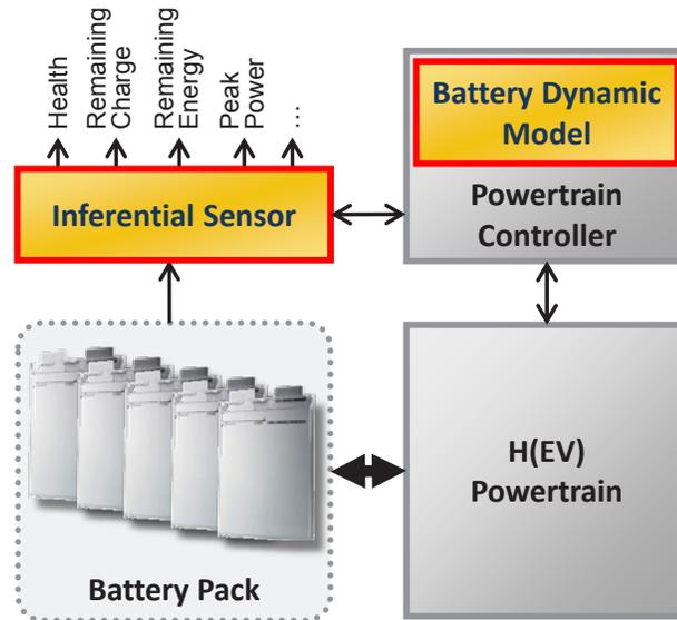
An inferential sensor for a Li-ion battery pack is needed for several variables in hybrid or electric vehicle powertrains.
