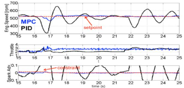
Disturbance rejection of MPC-ISC (blue) and conventional PID-based ISC (black) on a V8 engine. In this test, the AC compressor turned on after the power steering pump was already fully engaged. As a result, the spark authority was heavily reduced to avoid knocking, but MPC maintained control by adjusting the action on the throttle.
