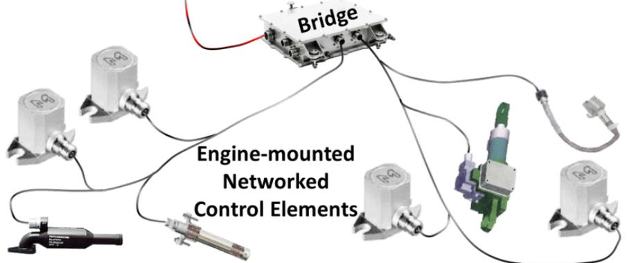
*Notional high-temperature, networked control elements remaining on the engine in a future distributed control architecture*
