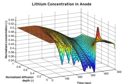
*Under high-current operation, high variation of lithium concentration on the anode surface (normalized diffusion depth of 0) creates "hidden waves" in the internal lithium concentration profile (normalized diffusion depth >0). Knowledge of the internal profile is essential for estimating parameters such as state of charge, but voltage measurements only reflect the surface concentration.*
