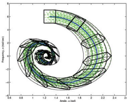
Illustration of phase angle (horizontal axis) and frequency (vertical axis) evolution in a power system showing nonlinear effects of parameter uncertainty. The complete uncertainty set generates a time-varying parallelepiped that is mapped along with the nominal trajectory (the blue curve).
