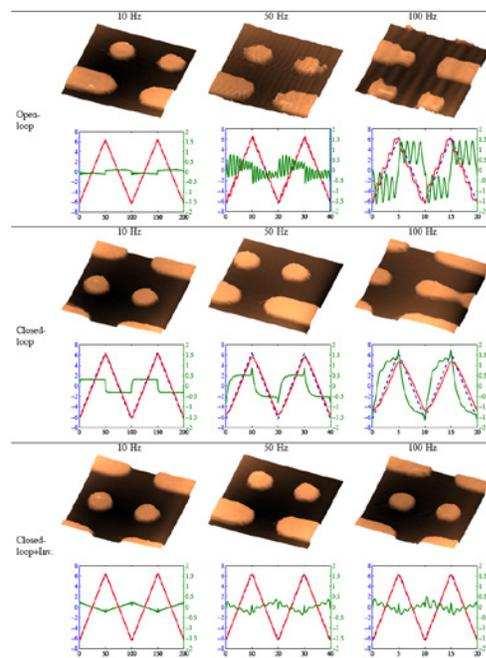
AFM scan results obtained at 10 Hz, 50 Hz, and 100 Hz in open-loop, closed-loop, and closed-loop with inversion-based feedforward. 3-D topography of the sample is plotted. The fast axis displacements ( $\mu\text{m}$  vs. ms) are plotted in red and tracking errors ( $\mu\text{m}$  vs. ms) are plotted in green. Reference signals are plotted in blue.
