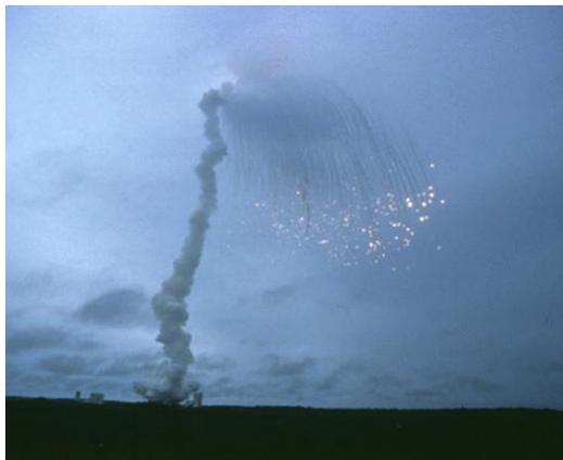
*During the Ariane 5 rocket's maiden flight in 1996, flight control software malfunctioned and the rocket had to be destroyed by remote command early in its trajectory. The malfunction was the result of improper reuse of Ariane 4 software. Hardware redundancy was no help since both computers ran the same incorrect software.*
