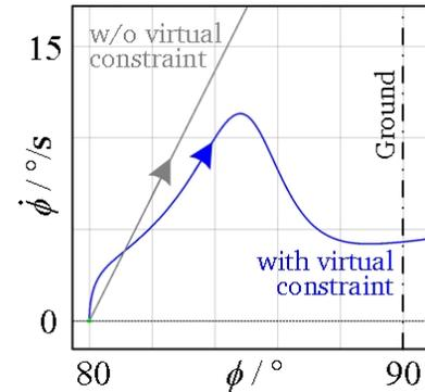
The transition from two wheels to all wheels in ground contact can be designed to achieve a soft landing using the “virtual constraints” framework. The upper-lower body angle ( $\rho$ , see figure below) and the lower body angle ( $\theta$ ) are coupled in the control system output function. The system zero dynamics of the SCD when falling to the ground are such that the upper-body motion causes a deceleration of the lower body as soon as the ground is close.
