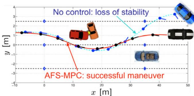
DLC with (black and white car) and without (blue car) MPC-based driver assistance that coordinates active front steering and differential braking. The test executed on a snowy road at approximately 50 kph shows that MPC helps the driver to enlarge the car operating envelope. (In both cars, electronic stability control was disabled for this test.)
