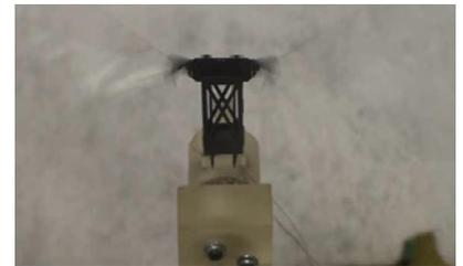
*Two piezoelectric actuators enable independent control of the motions of the flapping wings on this test vehicle.*
