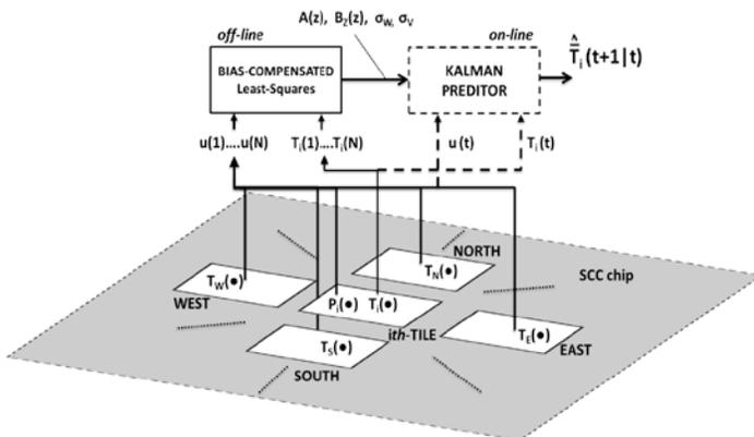
Distributed and robust thermal model learning strategy based on ARX-plus-noise system identification. The model takes as input the core power consumption and neighbors' core temperatures. It estimates the noise variance and the model parameters suitable for the Kalman predictor. The complexity of each single model is constant as the number of cores increases. Inputs to the Kalman predictor are also the current core power consumption and neighbors' core temperatures.
