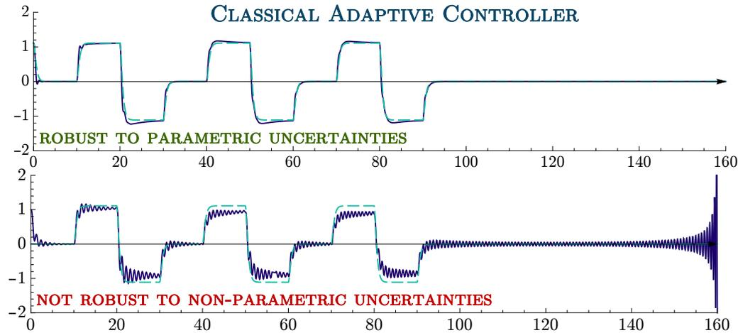
GOAL: FIND A CONTROLLER THAT ADAPTS TO PARAMETRIC UNCERTAINTIES AND IS ROBUST TO UNMODELED DYNAMICS – BOTH ARE INEVITABLE IN REAL-WORLD SYSTEMS
