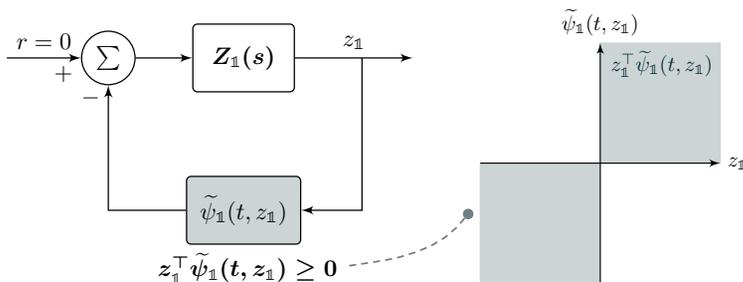
PERFORM LOOP TRANSFORMATIONS, AND ENFORCE A STABLE FEEDBACK INTERCONNECTION BETWEEN LINEAR SUBSYSTEM AND NONLINEARITY ISOLATED TO FEEDBACK PATH
